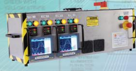
Custom Designed Portable Heat Treat System Ramp/Soak Temperature Controllers and other electronics are mounted in a custom sized portable stainless steel cabinet to power silicone rubber electric heating elements.
